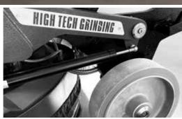
distinguished by a perfect balance of drive, motor and chassis. The powerful drive, designed without belts, ensures an ideal power flow and smooth operation, making this machine series exceptionally powerful. The machines
